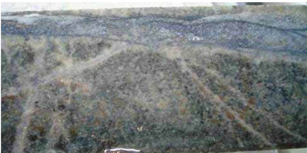
Anthony prospect - sawn drill core showing quartz-Mo vein cutting stockwork veins in altered granite. Hole RCD09-19, depth 226.2m
