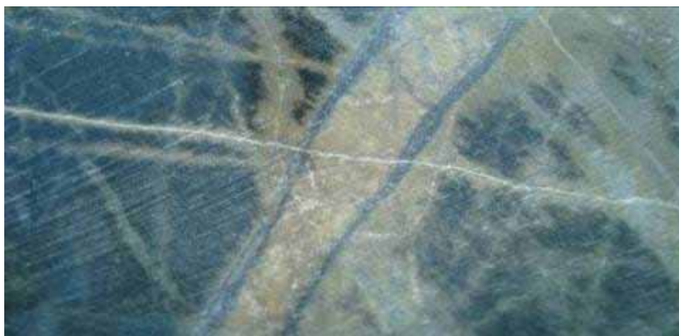
Anthony prospect - sawn drill core showing quartz-Mo veins in altered schist. Hole RCD09-19, depth 291.1m
