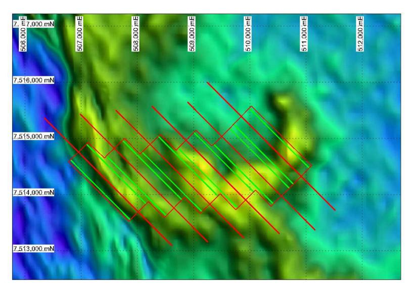
**Left:** Magnetic image showing a "high" (red) related to magnetic intrusive bodies, and surrounded by subdued negative magnetic anomalies (blue lines). White lines = potassium radiometric anomalies possibly indicating rock alteration. Previous shallow drilling near the edge of the magnetic anomaly intersected elevated base metals & gold (up to 2m at 2.0 g/t Au). The magnetic "low", possibly caused by rock alteration, has not been tested
