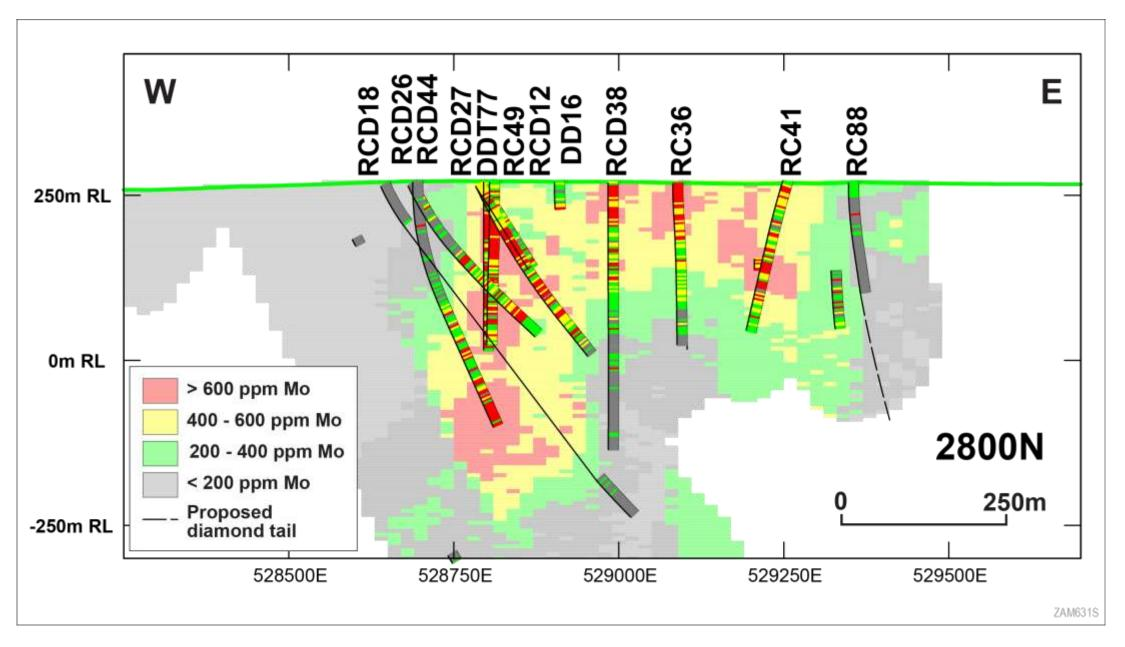
Drill cross-sections (west-east) through the Anthony deposit show high grade zones surrounded by lower grade mineralisation. Drill holes have intersected potentially ore-grade molybdenum mineralisation down to 500m depth below surface. The deposit shape is conducive to a large open-pit mining operation
