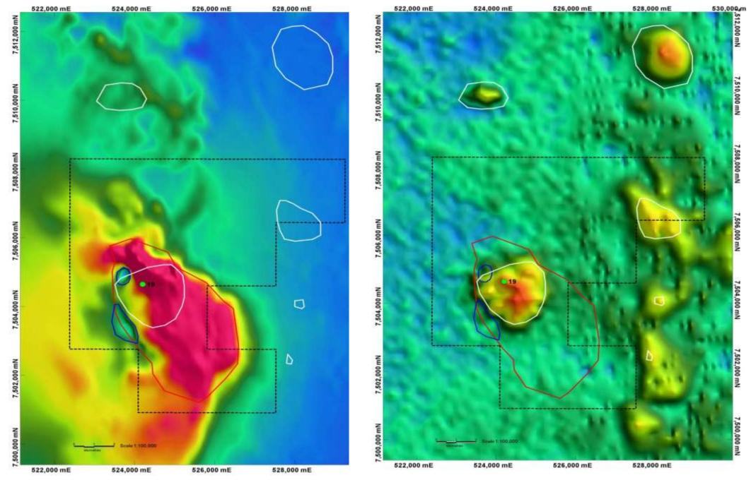
The target is an untested magnetic anomaly with a coincident potassium anomaly indicating an intrusive igneous complex. There has been no previous detailed exploration
