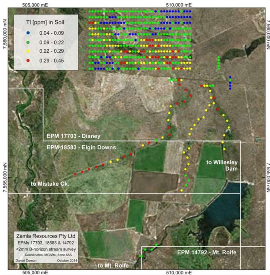
Figure 6. Assay results for thallium in drainage systems at southern Disney
