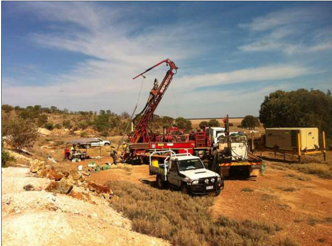
Figure 2. Mitchell Services RC Schramm 450 drill rig at Belyando
